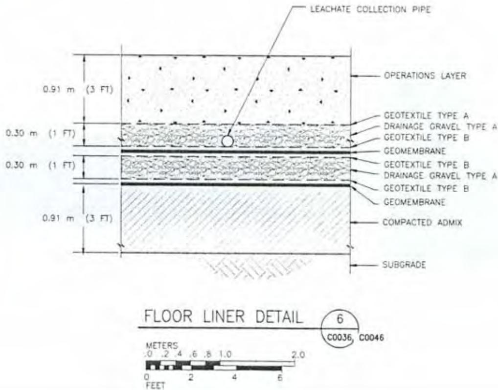
The liner was then constructed on top of the compacted sub grade. A schematic of the ERDF liner is shown in Figure 3.2.2.
