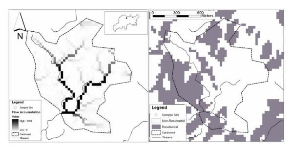
Figure 3. Catchment A, with a low raw spatial drainage index of 0.17.
