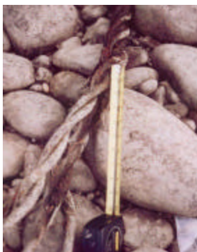
c. One-and-a-half inch steel cable.
