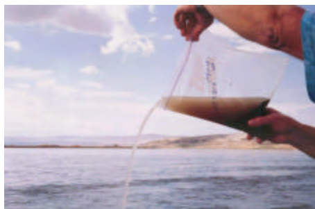
Fig.2.b. Pouring off suspended sediment fraction
